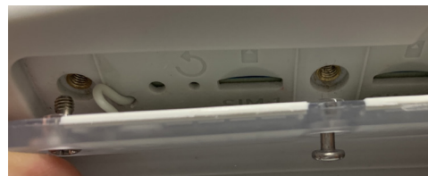
Incorrect tether placement
