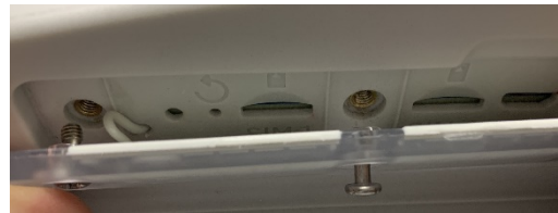
Incorrect tether placement
