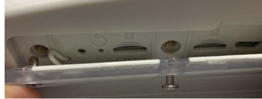
Incorrect tether placement
