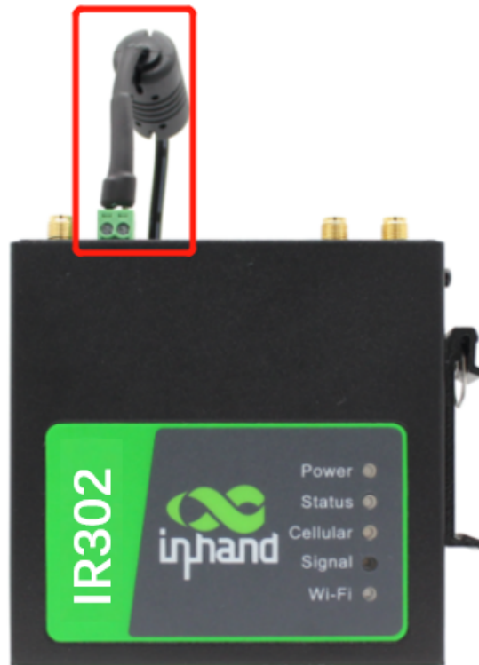
Fig. 4-5 Power Supply Installation
