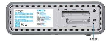
3. Press the SIM tool on the button for about five to six seconds, then your 5G Indoor Router will restart.
